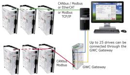
Drive control through commands by Master Controller. Suitable for multi axes systems (up to 127 drives). Built in powerfull Motion Module functionality assures perfect synchronization among axes and reduces Master Controller workload
